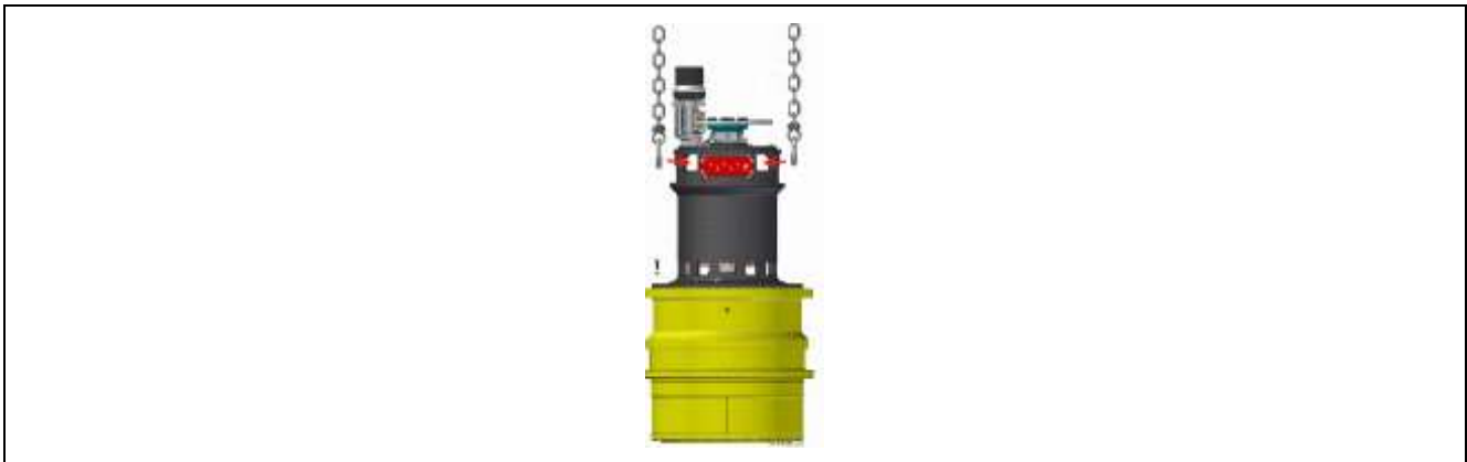
Figure 24. Planetary drive and traction motor positioned for motor removal
