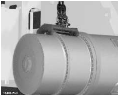
Figure 18. Crane attachment for removal of traction motor/planetary drive/assembly
