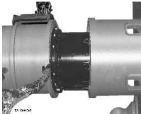
Figure 22. Hoisting assembly from axle
