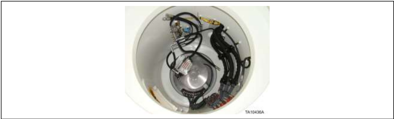
Figure 23. Typical view inside axle (some models have a different brake actuator than shown in photograph)
