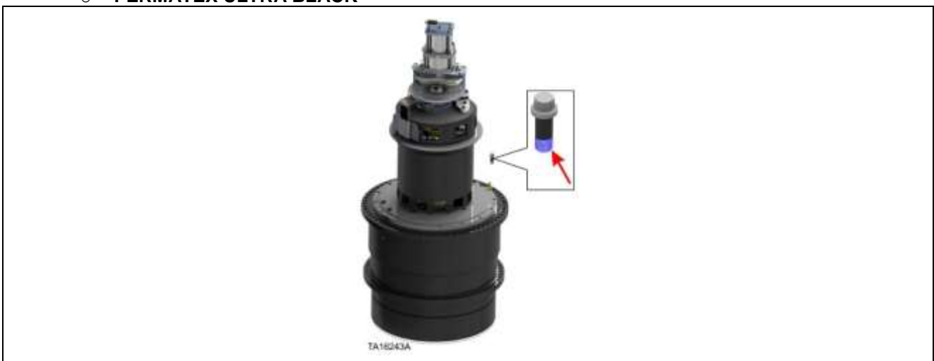
Figure 42. Apply sealant to all motor-to-planetary drive capscrew threads
