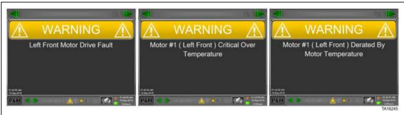
Figure 36. Examples of Yellow Warnings Associated with Motor Over-Temperature
