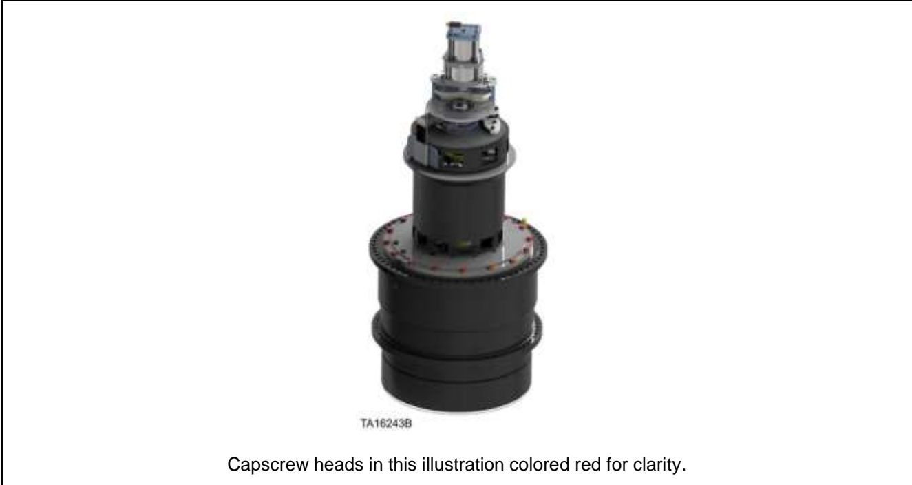
Figure 43. Install all motor-to-planetary drive capscrews
