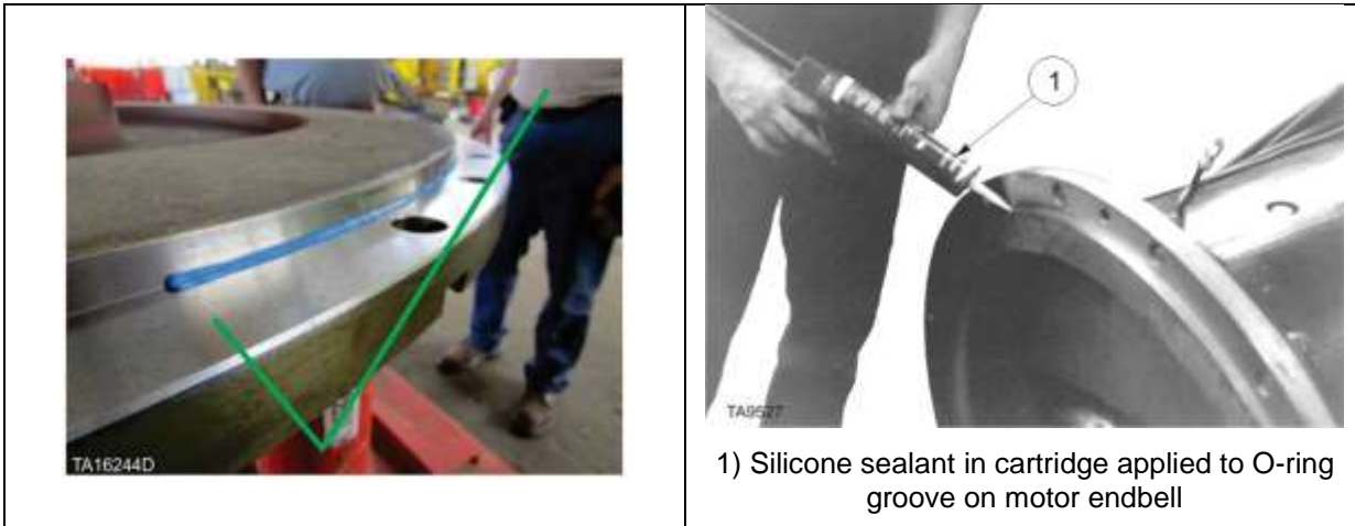
Figure 37. Correct application of silicone sealant
